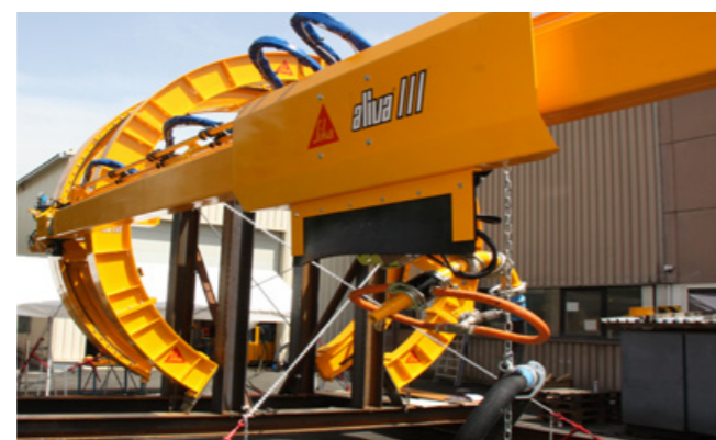
Spraying robot bridge-type system
