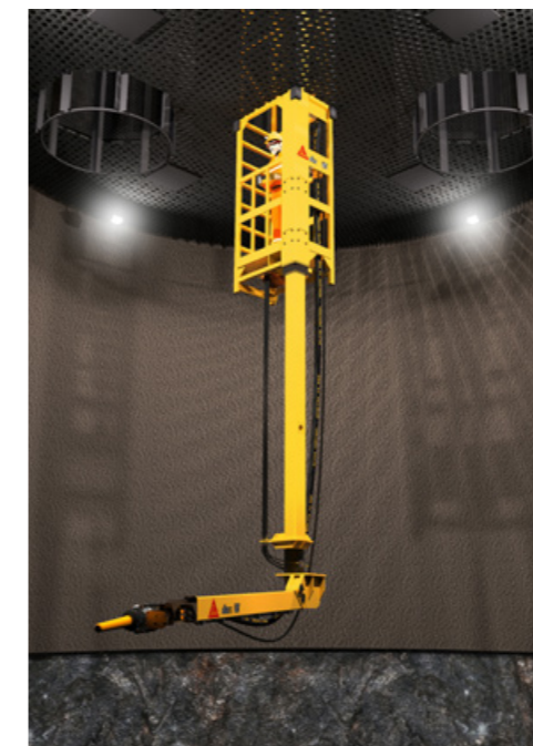
Shotcrete application 3m hub, 360° spraying angle
