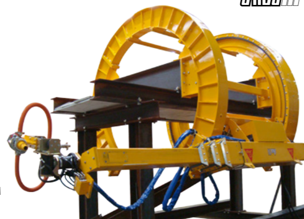
Spraying robot with telescopic spraying arm (This photo shows the set-up on a steel help construction)
